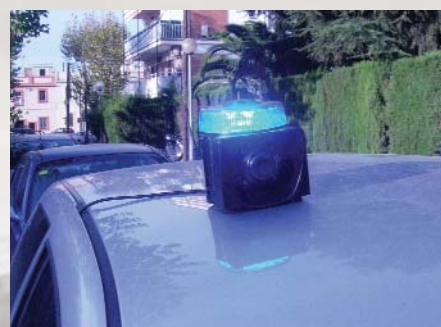
The new Federal Signal LM500 combination light and siren unit.
